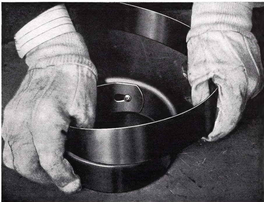
Figure 4—Winding Spring into Case
