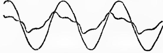
Fig. 91.—Oscillograph of transformer output.
